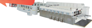
Full Servo Flexo Printer Slotter Die Cutter Inline Folder Gluer Counter Ejector (Top & Bottom Printer) 全伺服上下印刷开槽模切粘箱联动线
